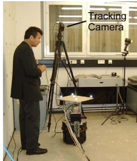
Figure 8. PLP-CAM robot and tracking camera
