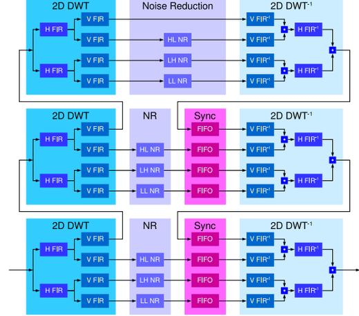
Figure 9. DWT based 2D noise reduction
