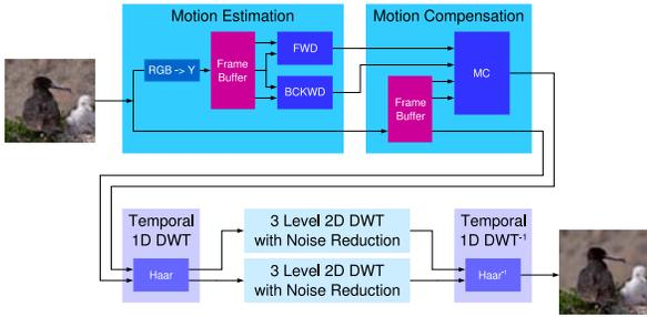
Figure 8. Advanced noise reduction algorithm
