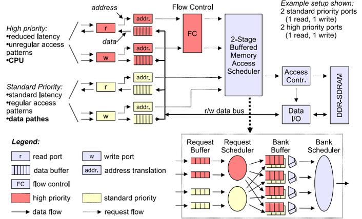
Figure 6. Memory Controller Block Diagram
