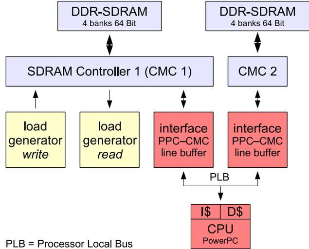
Figure 13. CMC QoS test environment
