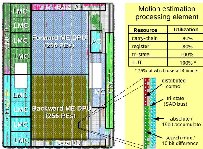
Figure 10. Mapping and resource usage in a Xilinx XC2V50P device
