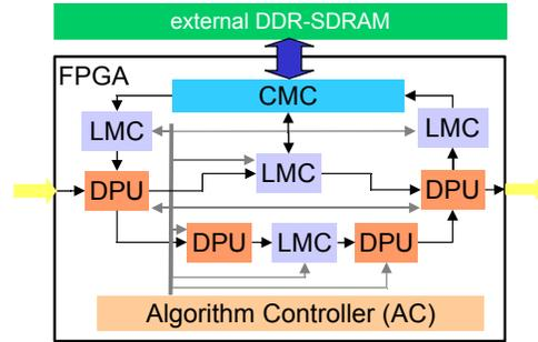
Figure 4. FlexWAFE Reconfigurable architecture
