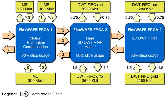
Figure 12. Algorithm mapping
