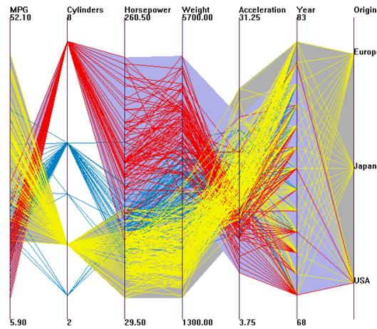
■ **Figure 1** Two hyper-boxes in Parallel Coordinates. Two clusters have been isolated based on the second dimension. The brown and grey regions indicate the surrounding hyper-boxes for the clusters. Image generated with XmdvTool [6, 11].
