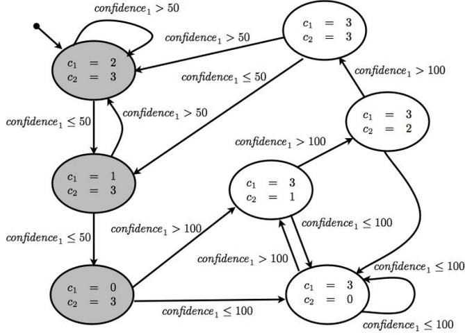
**Fig. 2.** State Transition Diagram for Adaptation Behaviour of Module 1
