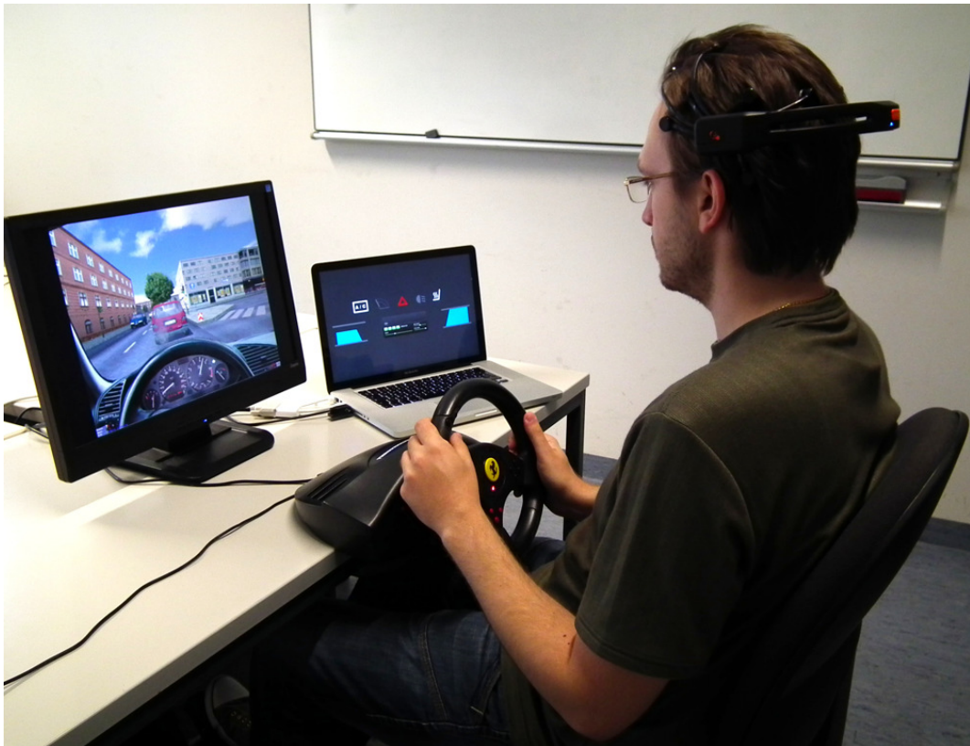
■ Figure 1 Image of a participant while interacting with the driving simulator and the EEG-controlled dashboard.
