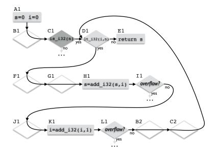
**Figure 5** Control flow graph of **sum** function transformed by basic block versioning.
