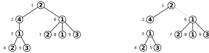
■ Figure 1 Left: A weighted tree t . The small numbers next to the nodes denote their IDs. The trace of a depth-first-traversal of t is 241223314122113312, where we ambiguously write w for (\text{'d'}, w) and \bar{w} for (\text{'u'}, w) . Right: Partitioning of t into three parts with bottleneck value 7. A streaming algorithm should output the IDs of the root nodes of the created partitions. Here, these are 1, 3, 6.
