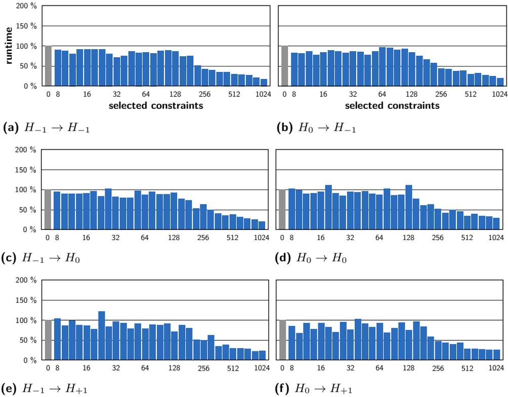
■ **Figure 3** Runtimes after generalized constraint feedback with varied horizons. In setting  $H_x \rightarrow H_y$ , constraints were extracted and generalized with benchmark set  $H_x$  and reused for solving  $H_y$ .
