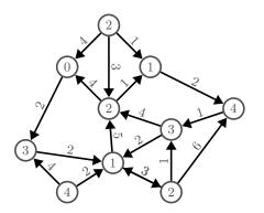
(a) An instance containing a directed graph with capacities on the vertices and weights on the arcs.
