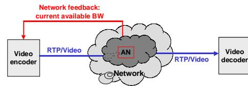
Fig. 1. Network-based rate-control
