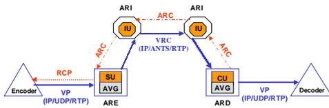
Fig. 2. The Active Regulation Mechanism architecture
