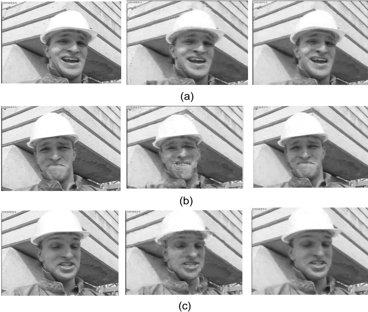
Fig. 8. Comparison of the ARM with the RTCP Best-Effort. (a)The 16th frame, in the left the original frame, the middle is the RTCP environment (21.05dB) and in the right the ARM (22.63dB). (b)The 40th frame. the proposed algorithm without loss (22.69dB): prediction of loss appear in the middle (RTCP 16.87dB). (c)The 76th frame, in the middle the RTCP correction (23.43dB) and in the right the ARM correction (30.55dB)
