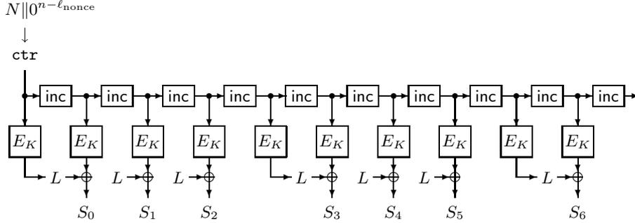
**Fig. 2.** Illustration of the keystream generation algorithm. This example uses  $w = 3$  and outputs  $l = 7$  blocks of keystream  $S = (S_0, \dots, S_6)$ .
