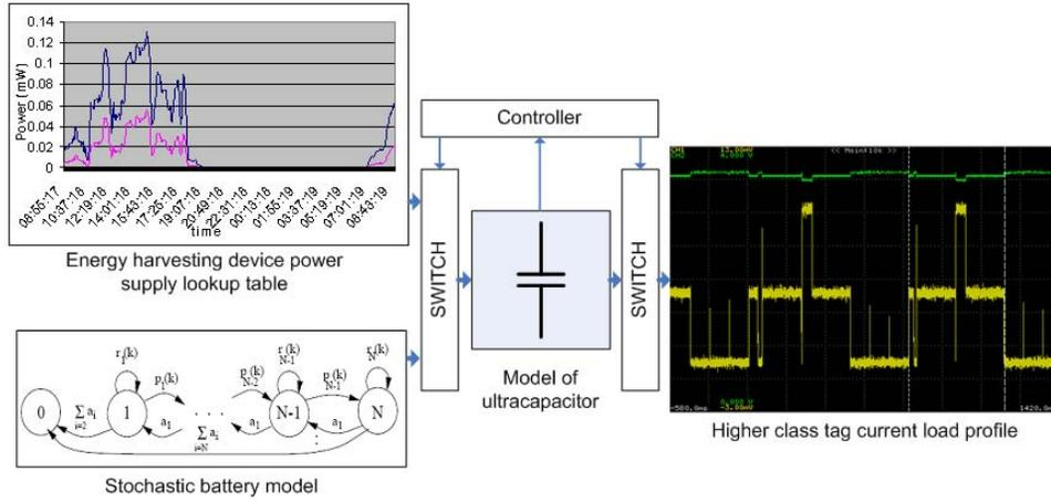
**Fig. 9.** Basic blocks of the simulation model
