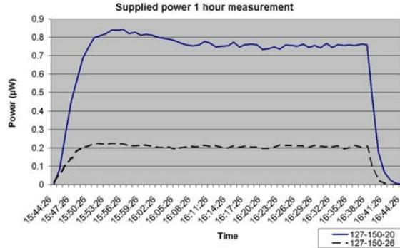
**Fig. 4.** Measurement of the power supplied by a thermo generator - 1 hour
