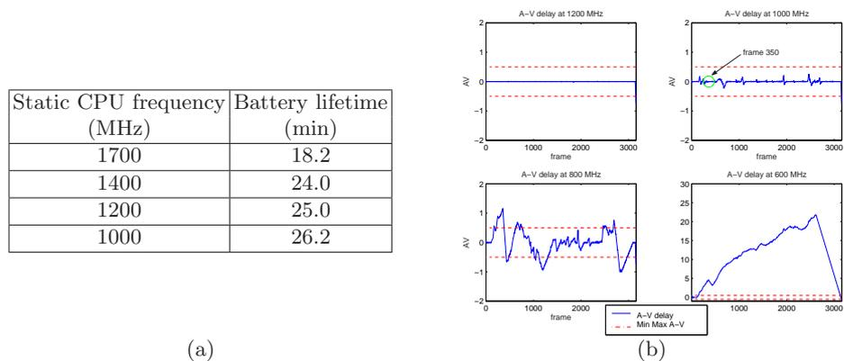
**Fig. 2.** a) Battery lifetime in minutes when playing the Jarhead video at various CPU frequencies. b) Per-frame execution time for the video Jarhead at various CPU frequencies.
