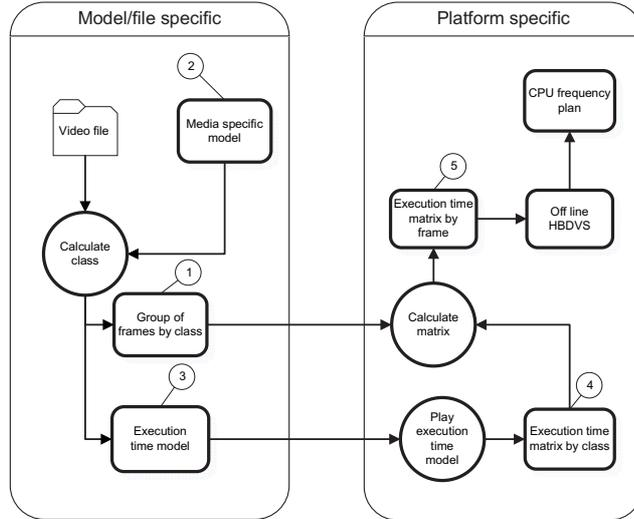
**Fig. 3.** The CbDVS algorithm
