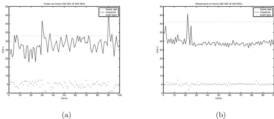
**Fig. 1.** Average treatment time, in milliseconds, for 100 frames of the (a) Fedex and (b) Mastercard insert codes videos on a Via C3 running at a CPU frequency of 800 MHz. The frame time is indicated by a dotted horizontal line in each graph.
