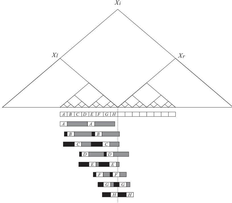
**Fig. 3.** Illustration of Lemma 5 for height  $h = \text{height}(|X_i|) - 5$ . No repetitions  $zz$  hinged on variable  $A$  can touch or cover the boundary of  $X_i$ , since repetitions  $zz$  are hinged on variable  $A$  only if  $2 \times |A| - 1 = 2^h - 1 \leq |z| < 2^{h+1} - 1 = 4 \times |A| - 1$ .
