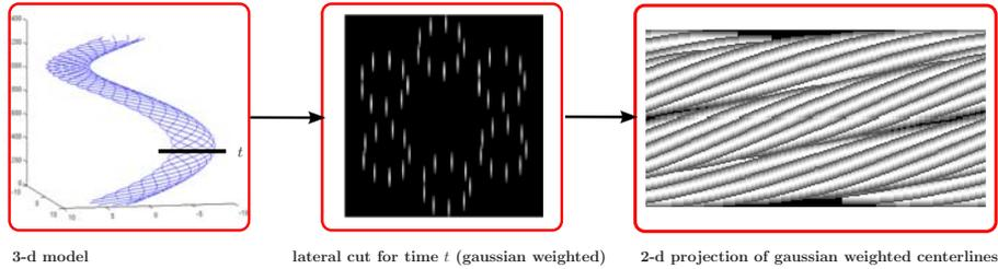
**Fig. 1.** Pipeline which projects 3-d wire centerline model to 2-d image plane.
