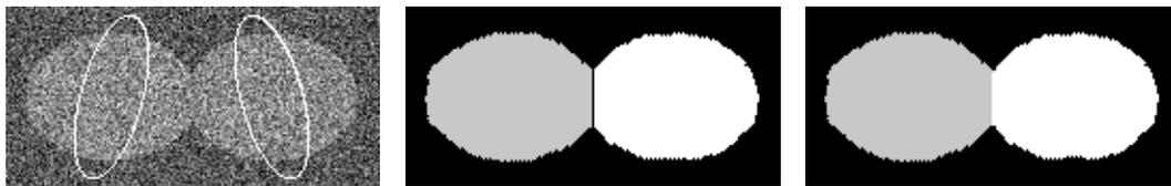
■ **Figure 3** Segmentation of touching objects ( $\mu = 0.5$ ,  $\lambda_1 = \lambda_2 = 1$ ). Left: Input image overlaid with two initial contours. Centre: Segmentation result of the SP algorithm. Right: Segmentation result of the RI algorithm.
