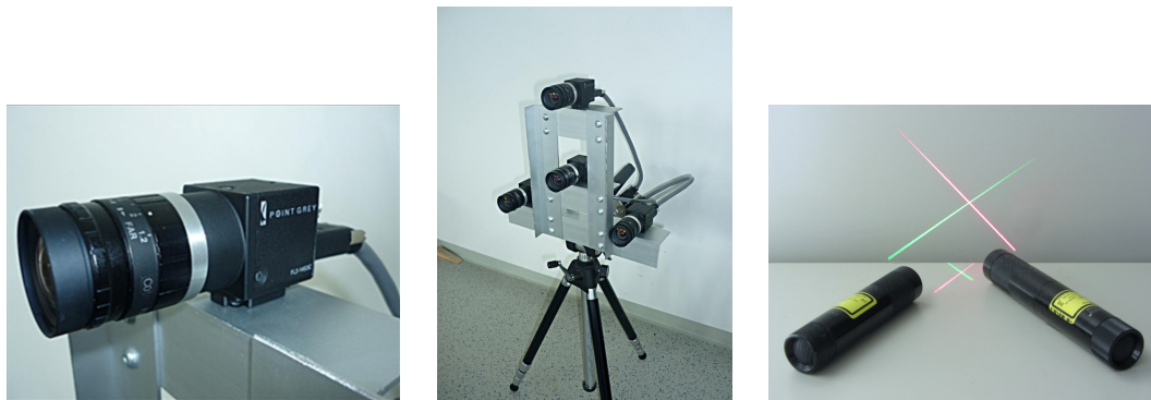
■ Figure 1 A system of four Point Grey Flea ® 2 FireWire 800 cameras (left) arranged in an upside down Y-constellation (middle). Red and green line-laser probe (right).
