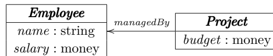
■ Figure 3 The model EP in the simple modelling language consists of two classes with attributes and a function between them.
