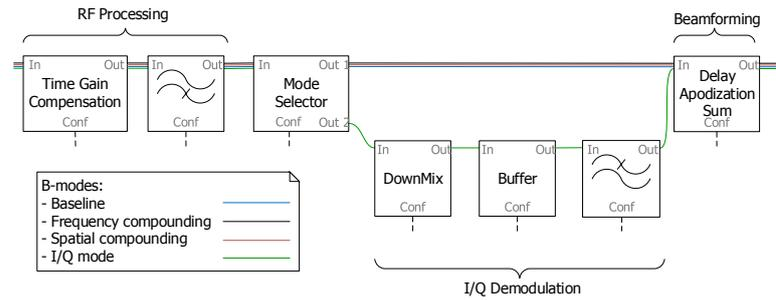
■ **Figure 10** RF Processing, Demodulation(I/Q mode), Beamforming.
