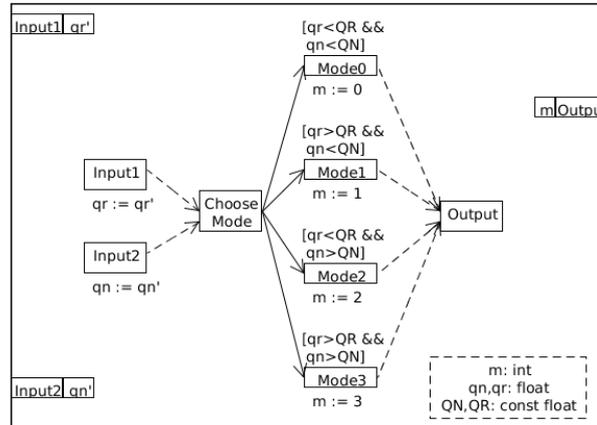
■ **Figure 13** Simple QoS controller as well-triggered component.
