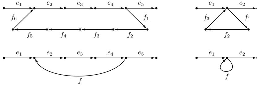
■ **Figure 1** Examples of walks  $e_1 \cdots e_\ell$  which are not omnitigs, due to the existence of a path  $p$  satisfying the conditions of Definition 1. In the first row,  $p = f_1 \cdots f_{|p|}$  with  $|p| > 1$ . In the second row,  $p = f$ . In the left column,  $p$  is a non-empty open path. In the right column,  $p$  is a closed path.
