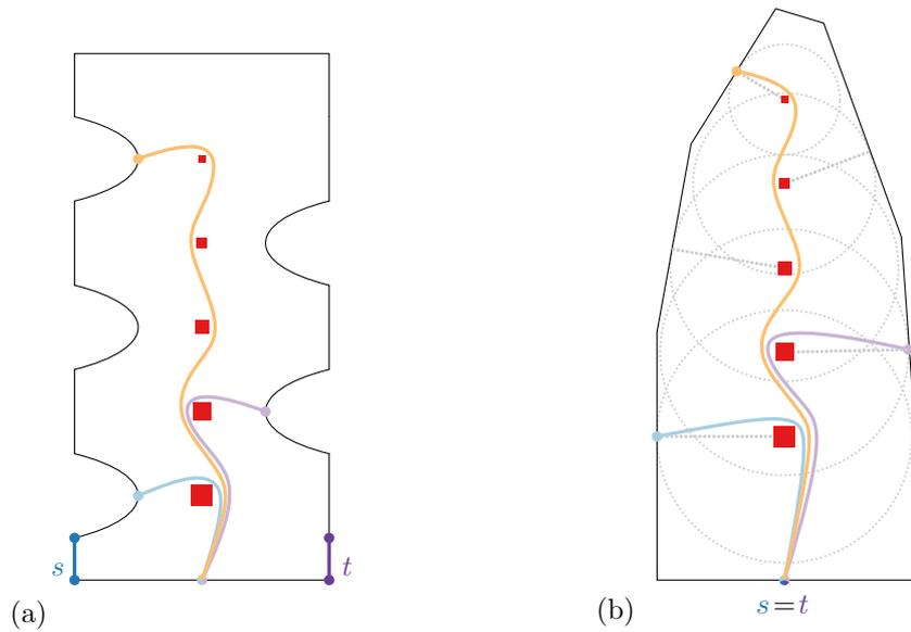
■ **Figure 4** (a) A leash may need many inflection points in the variable-weight case. (b) The same principle in the convex case, with one boundary path and the two initial leashes collapsed to a point. Closest point and corresponding distance circles indicated for each obstacle.
