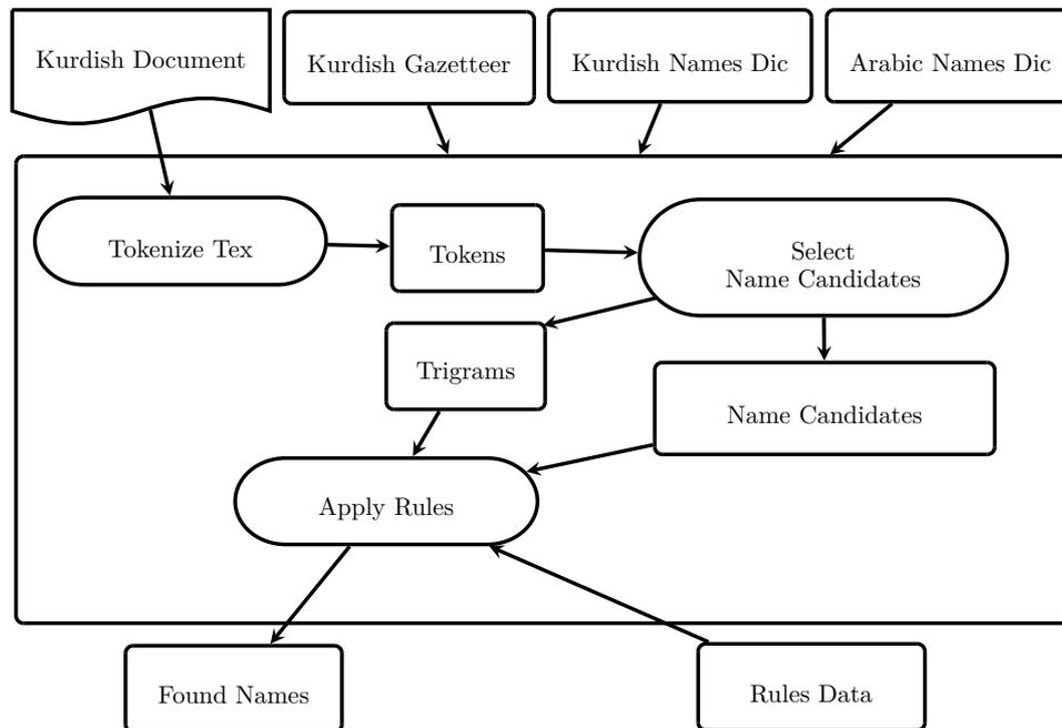
■ **Figure 1** Kurdish PNR Architecture - The architecture is based on three dictionaries and a set of rules which is used by the internal part of the system to find out the Proper Names.
