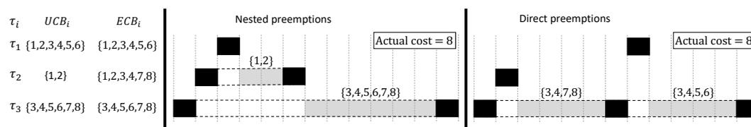
■ **Figure 1** Example of the pessimistic CRPD estimation in both, UCB- and ECB-union based approaches. Notice that the worst-case execution time (black rectangles) is in reality significantly larger than CRPD, but the focus of the figure is rather on preemptions and CRPD depiction.
