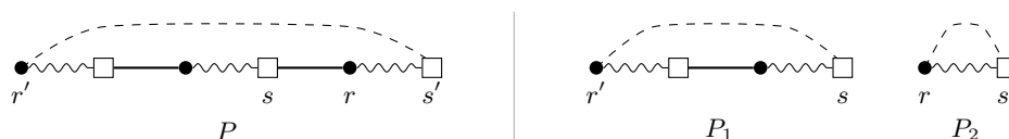
■ Figure 3 Illustration of Step 4 in Algorithm 1. Edges of M^* are snaked, edges of M^F solid and edges of M \setminus M^F dashed. After unfreezing r , the removal of (r, s) splits the path in M^* \oplus M^F in two parts.
