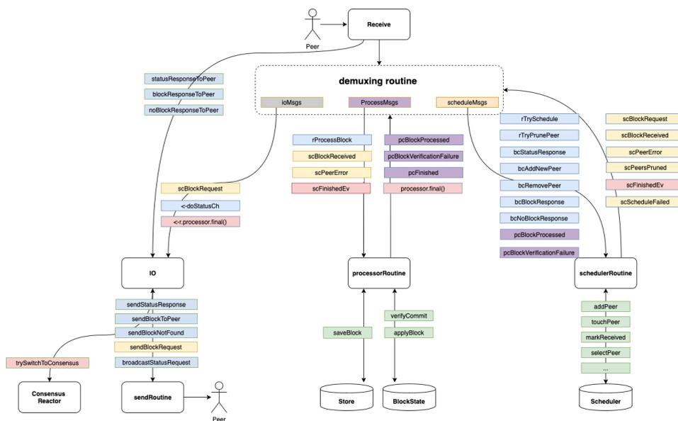
■ **Figure 2** Concurrent threads of execution in the FastSync implementation [13].
