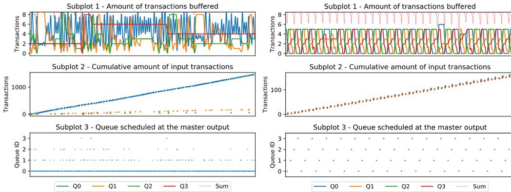
(a) FP with ordering  $C_0 \succ C_1 \succ C_2 \succ C_3$ . (b) TDMA with slots of 256 clock cycles.
