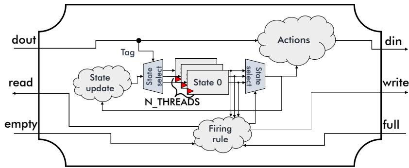
**Figure 7** Schematic of an actor supporting tagged tokens. The combinational logic **Firing rule** must consider only matching tokens. Combinational logic, **Actions** and **State updates**, is shared, while the sequential one **State** is replicated for each supported thread.
