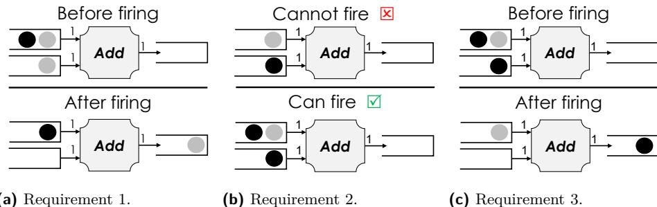
**Figure 3** Representation of the three requirements using the *Add* actor, whose token rates are indicated on the arrows. In each image, the status of input and output buffers is depicted using different colors for tokens belonging to different threads.
