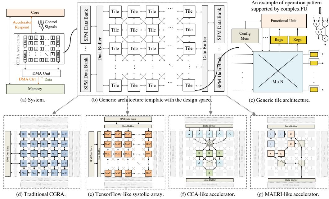
**Figure 3** Generic architecture template – The generic parameterizable template provides a design space to be explored and eventually generates an optimized accelerator for the given workloads. (d)-(g) show how the template is customized into different state-of-the-art spatial reconfigurable accelerators.
