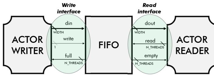
**Figure 4** Schematic of the connection between a FIFO and two actors using the `write_interface` and the `read_interface`. `WIDTH` is the sum of `DATA_WIDTH` and the tag width, which is  $\log_2(N\_THREADS)$ .
