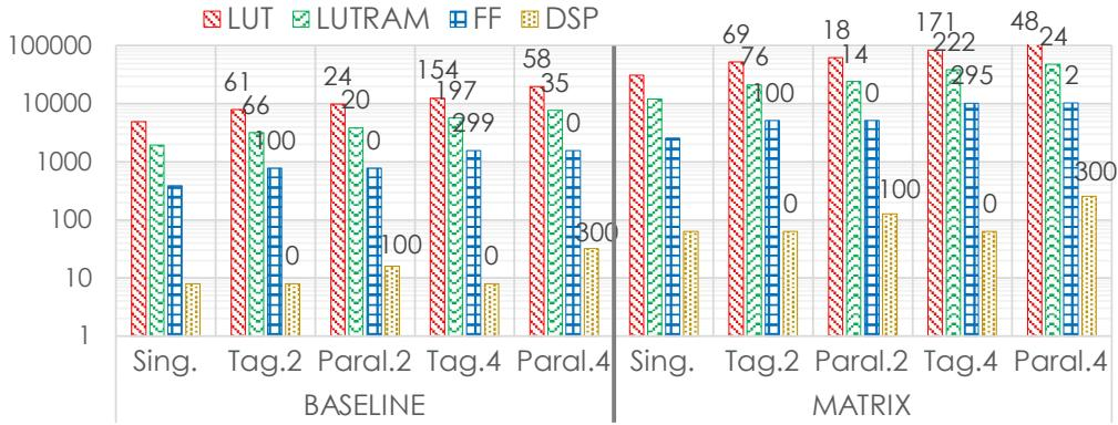
**Figure 10** Resource utilization of all the accelerators described in Sect. 4.1. Data are reported on a logarithmic scale. On top of Tagged columns percentage variation referred to Single, and on top of Parallel columns percentage variation referred to the corresponding Tagged one.
