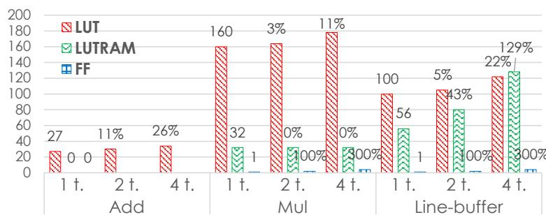
**Figure 9** Resource utilization of Add, Mul, and Line-buffer actors supporting 1, 2, or 4 threads. On the 1-thread columns the absolute value is reported, on the others the variation with respect to that one.
