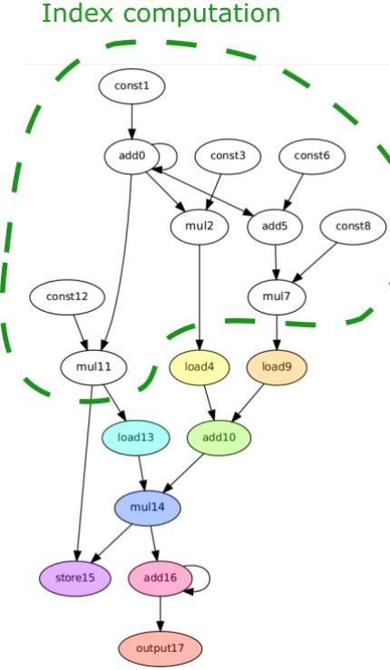
**Figure 4** Original accumulator DFG generated by the CGRA-ME framework versus the proposed accumulator DFG. The proposed DFG discards all the nodes for computing the index and replaces them for attributes (e.g., initial address and stride) to configure the inputs/outputs nodes.
