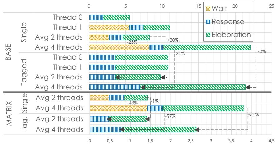
**Figure 11** Time performance with same-size elaborations. Thread 0 and Thread 1 are the evolution of the threads when 2 of them are elaborated. Avg 2 threads and Avg 4 threads are the average time performance when respectively 2 or 4 threads are considered. Arrows show the percentage variation in the Tagged accelerators compared with the corresponding Single ones. Timescales are in us.
