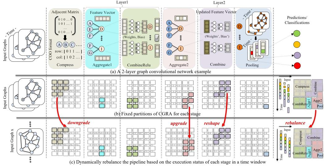
**Figure 5** Example of dynamic rebalancing – (a) A 2-layer GCN inference includes 6 kernels. (b) Fixed partition for each stage targeting high throughput. (c) Dynamically reconfigure the CGRA based on the execution status of each kernel, which rebalances the pipeline and improves the overall throughput.
