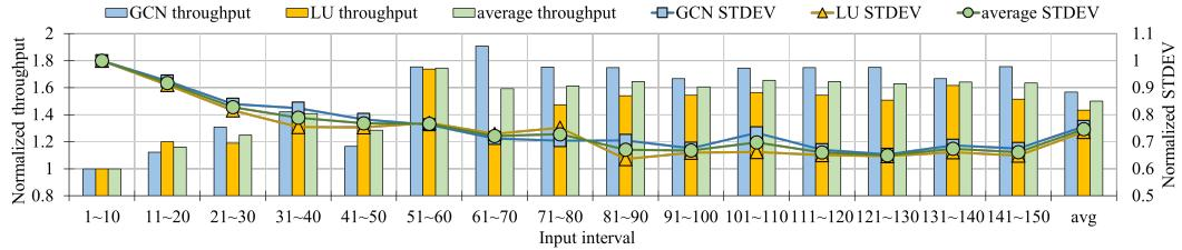
**Figure 7** Normalized throughput and normalized standard deviation of different applications running on our reconfigurable designs over the baseline – The time window has a size of 10 rounds and the SPM memory is 32KB.
