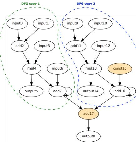
**Figure 6** Accumulate DFG with a loop unrolling factor of two.
