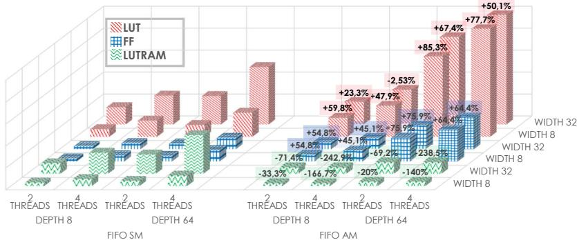
**Figure 8** Resource-utilization comparison between the Separated-memory FIFO (on the left) and the Address-memory FIFO (on the right) varying design parameters:  $N\_THREADS=\{2, 4\}$ ,  $DEPTH=\{8, 64\}$ ,  $DATA\_WIDTH=\{8, 32\}$ . On top of the right-side columns the percentage variation with respect to the corresponding left-side column is reported.
