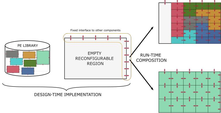
**Figure 2** Tile based composition approach. At design time (left) it is necessary to implement a library with different PEs and an empty reconfigurable region that only defines the interconnection with the rest of the system. At run time (right) different accelerators can be composed on the fly by stitching together PEs from the library.
