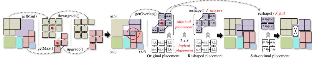
**Figure 6** The *upgrade()*, *downgrade()*, and *reshape()* operations form the logical placement by enabling appropriate interconnection between neighboring tiles.
