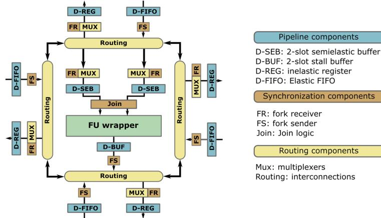
**Figure 3** Baseline PE architecture. The PE is divided into four different components. In blue are the Data-Driven Pipeline Unit (DDPU), in yellow the routing elements, in brown the synchronization components and in green the FU. Figure extracted from [4].
