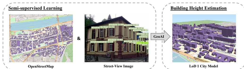
■ Figure 1 An overview of building height estimation via semi-supervised learning from OpenStreetMap data and street-view images.
