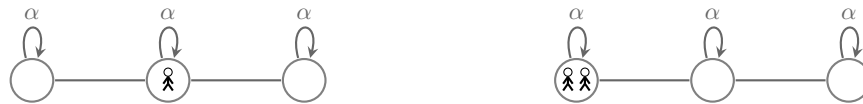
■ Figure 2 The Markov chain given by Efremenko and Reingold [7]. The cover time for the single random walk equals \frac{5}{1-\alpha} , while the cover time for the two random walks starting from any endpoint is \frac{2.25}{1-\alpha} + o(1/(1-\alpha)) , as \alpha \rightarrow 1 .
