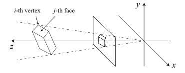
**Figure 2** Object and its projection.
