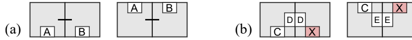
■ Figure 1 The black lines between two tiles indicate unique unimportant \tau -strength bonds. If \tau = 2 , str(A) = 1 and str(B) = 1 , then the two assemblies in (a) are \tau -combinable, since str(A) + str(B) \geq \tau and the positioned assemblies may be translated such that the A and B glues are aligned – such a combination is termed cooperative binding , since neither the A nor B glue are alone sufficient to satisfy \tau -combination. In (b), we consider two cases concerning the negative strength glue X . If \tau = 2 , str(C) = 2 , and str(X) = -1 , then the assemblies in (b) are not \tau -combinable since str(C) + str(X) < \tau . If \tau = 1 , str(C) = 2 , str(D) = 2 , str(E) = 1 and str(X) = -1 , then the assemblies are \tau -combinable since str(C) + str(X) \geq \tau ; however, the resultant assembly is unstable, since a cut along the X and E glue has strength str(X) + str(E) < \tau ; this violates the valid growth-only system definition.
