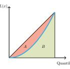
**Figure 1** The Lorenz curve is plotted in blue. The green area is  $B = \int_0^1 L(t)dt$ . The Gini coefficient is then G = 1 - 2B = 2A.
