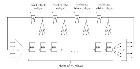
Figure 11 Overview of the whole construction, with one branch shown in detail. Rechargeable relays (RR), Recharging systems (RS), AND gates (A), Joins (J) and Forks (F) are explicitly shown.
