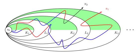
**Figure 9** Updates of the extra mode bit along runs  $\pi_1, \pi_2$ , drawn in blue while the memory-bit is one and in red while the bit is zero. The run  $\pi_2$  violates SEQ and is drawn as a dotted line once it does. Upon entering the green zone of  $K_i \setminus K_{i-1}$ , the runs attain the local objective  $\varphi_i$  and flip the mode bit.
