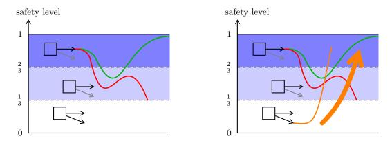
**Figure 8** Left: Starting from a state with safety level at least  $\frac{2}{3}$  the probability of keeping a safety level of at least  $\frac{1}{3}$  forever is at least  $\frac{1}{2}$ . Right: For the states with safety level less than  $\frac{1}{3}$  we aim at reaching safety level at least  $\frac{2}{3}$ .
