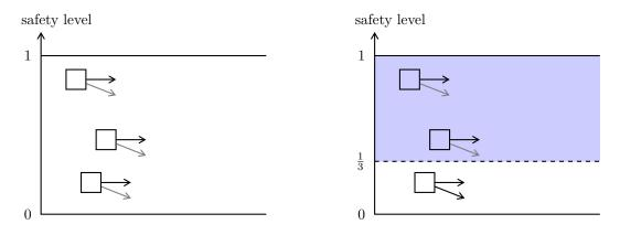
**Figure 7** Left: In this diagram the controlled states are arranged according to their safety level. A safety strategy entails not to pick successor states with smaller safety level, so grey transitions are not used. Right: The optimal safety strategy  $\sigma_{safe}$  is fixed for the states with safety level at least  $\frac{1}{3}$ .
