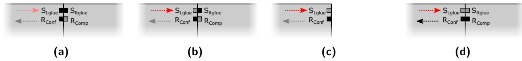
■ Figure 15 An example which verifies completion of an “off” signal. (a) An off signal is fired from another glue in the STAM tile. Notice that an off signal is denoted by a red arrow. (b) Upon signal execution, the S_{Lglue} turns off. (c) This causes the right STAM tile to detach. (d) A new tile may now attach, sending a signal which confirms that the S_{Lglue} has successfully been turned off.
