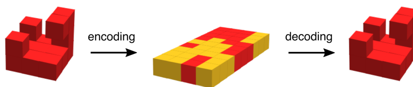
■ Figure 1 Schematic depiction of shape replication: (Left) An input assembly, (Middle) The assembly resulting from the encoding process which deconstructs the input assembly and encodes its shape, (Right) The assembly created by the decoding process, which uses the encoding as its input.
