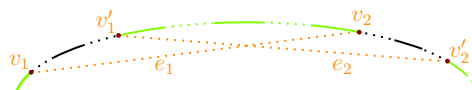
■ Figure 1 A skip formed by two non-matching edges e_1 and e_2 (in orange). Matching edges are represented by full lines and non-matching edges by dotted lines. The paths removed by the skip are depicted in black.
