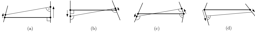
■ Figure 3 Two edge events and two vertex events where the feasibility of a top unit chord C (thick segment) changes for \theta increasing from \theta_1 in the interior of an interval of \mathcal{I}(O) . Assume \theta_1 = 0 . Each acute angle is marked with a circle. (a) An edge event where C becomes infeasible. (b) An edge event where C becomes feasible. (c) A vertex event where C becomes feasible. (d) a vertex event where C becomes infeasible.
