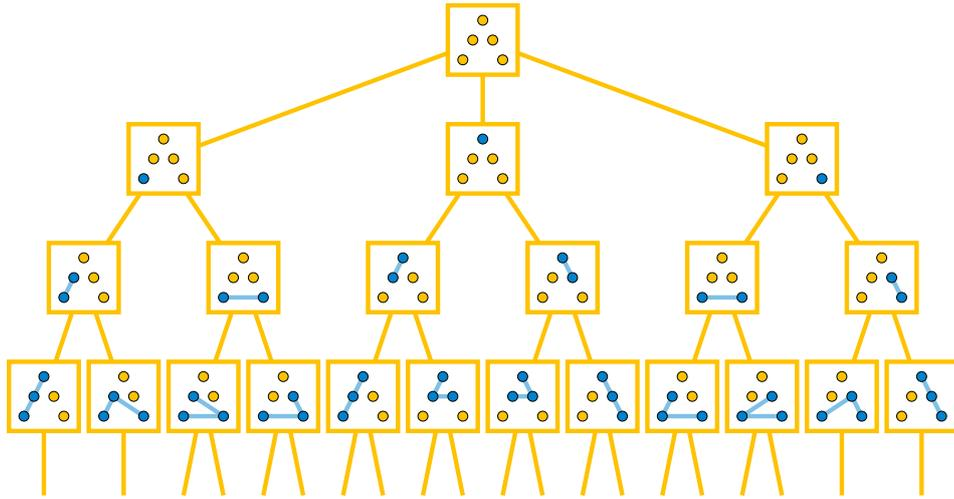
■ **Figure 2** A tree of the visible-vertex paths in a point set, where the parent of each path is obtained by removing its last point. This point set has  $\text{OFFLINE}(S) = 2$ . The root and the next two levels of nodes each have multiple children, but some nodes on the last level shown in the figure have only one child, because the last point on the path is collinear with all remaining points.
