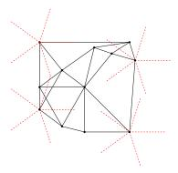
**Figure 1** Yao graph for ten points and k = 5 cones. The five cones are illustrated as red dashed lines around four example points.
