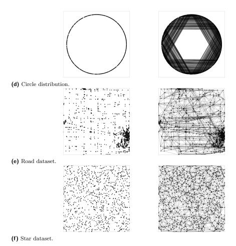
**Figure 10** Input distributions for n = 1000 points and resulting Yao graph for k = 6. For the grid distribution, the resulting graphs from exact constructions and inexact constructions are shown.
