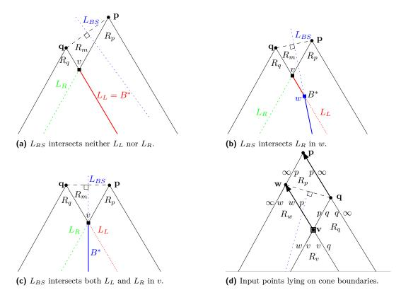
**Figure 3** Illustration of the three possible configurations for boundary  $B^*$  following an intersection point event. In all examples input point p is swept before q. Lines  $L_L$ ,  $L_R$  and  $L_{BS}$  are dotted, the resulting boundary  $B^*$  is denoted in bold. In Figure d), Yao graph edges are shown as bold arrows.
