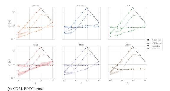
Figure 12 Algorithm runtime experiments. Experiments over varying input sizes are performed with k=6 cones. The gray line represents the time limit of 30 min per algorithm.
