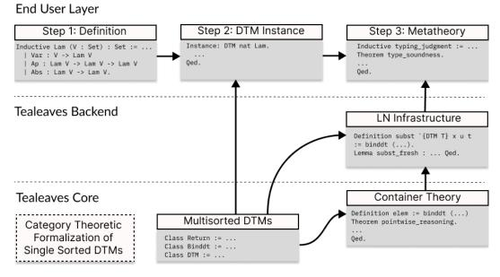
**Figure 6** Simplified Tealeaves architecture and user workflow.
