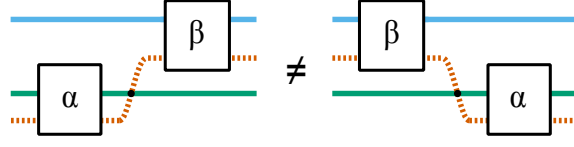
■ Figure 6 In the free premonoidal category over a monoidal graph, generators are augmented by a string on a new object called the runtime (dashed red). This prevents interchange (cf. Figure 1).
