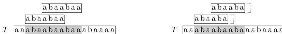
■ Figure 2 Left: the locus v of C = \text{abaabaa} in CST(T) is an explicit node and we have cv(v) = 10 , nov(v) = 1 (see Figure 1). Right: the locus v' of the prefix C' = \text{abaaba} of C is an implicit node one character above v . We then have cv(v') = cv(v) - nov(v) = 9 .
