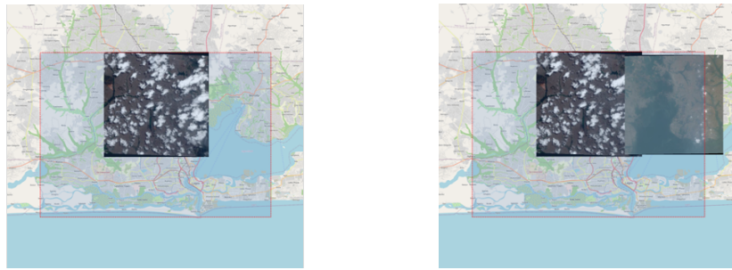
■ Figure 2 A cloudy region of an image can be covered by a non-cloudy region of another image, impacting the cloud coverage percentage of the final mosaic.
