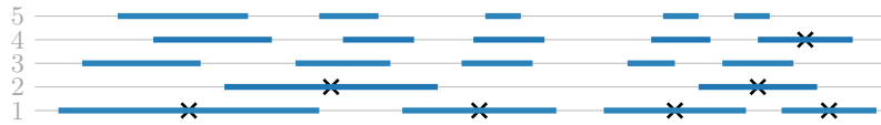
■ Figure 2 A set of intervals and a coloring produced by the 2-approximation algorithm. The intervals that lie in M(\mathcal{I}) at the top level of the recursion are marked with crosses.
