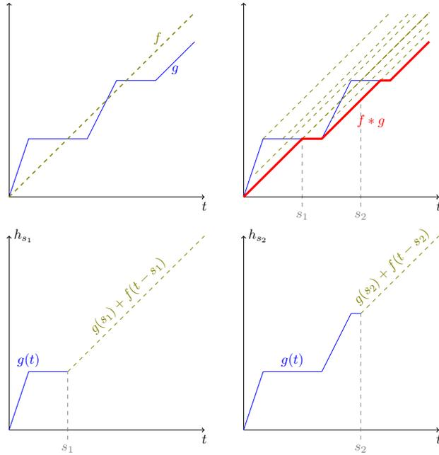
■ **Figure 10** Top: Illustration of the convolution ( $f * g$ : thick) between  $f$  (dashed) and  $g$  (plain), from [2, Fig. 2.1]. Bottom:  $h_s : t \mapsto g(t \wedge s) + f([t - s]^+)$  for two specific values of  $s$ .
