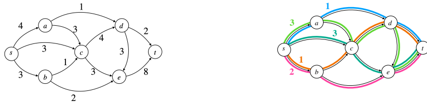
(a) A flow network. (b) A flow decomposition into paths of weights (1, 1, 2, 3, 3).
