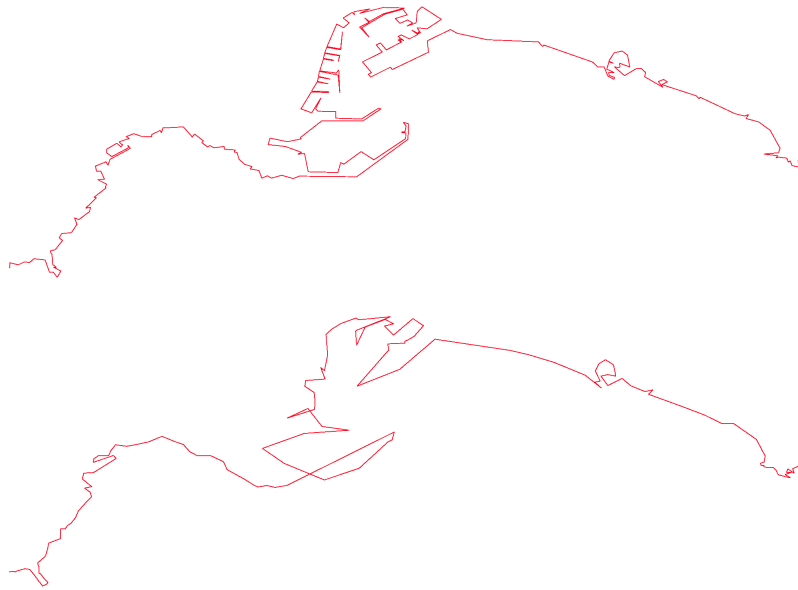
■ Figure 8 Comparison of GLS based simplification (top) with naive subsampling (bottom) on the port of Mallorca instance using 4382 points each. In the bottom image, shape distortions and visual artifacts are clearly visible.
