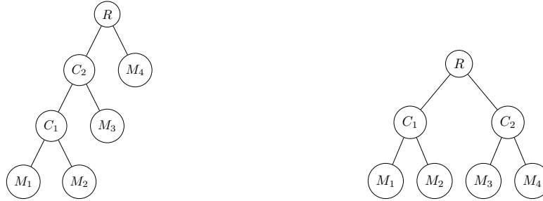
(a) Imbalanced contraction tree for the order jkl . (b) Balanced contraction tree for jl k and ljk .
