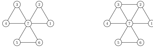
■ Figure 2 Examples of admissible subgraphs of \mathcal{G}_{\text{wheel}}(6) . On the left is a friendship graph in which every non-center node has degree 2, and on the right is a subgraph where every non-center node has degree 2 or 3.
